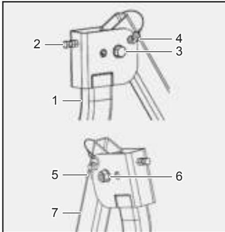
1. Loosen the bolt (3) and nut (6) of the frame. (Do not unscrew them completely.)
