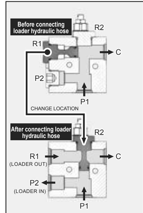
When installing a loader, the plug of the port R1 should be fit to the port
