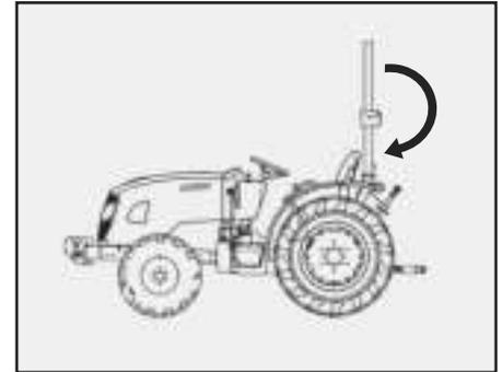
3. Fit the pins (5) through the holes of the frames (1 & 7) and fit the snap pins (4) into the holes of the pins (5) to fix the frames.
